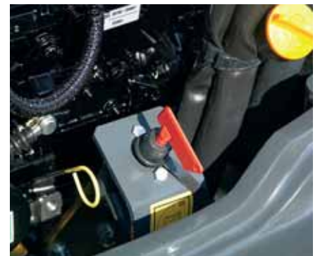
The battery main switch is standard
