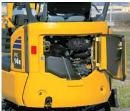
Rear bonnet: quick engine check and fuel tank refilling
